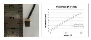
Over 50 stacking of single crystal which is small size and large displacements for actuator such as 'Deformable Mirror'. (6.7um@100V)
