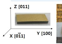
A single crystal 2-2, 1-3 composite element which is small, lightweight and conformal to hull shape for hydrophone and communication receiver on UUV or AUV or on a submarine.
